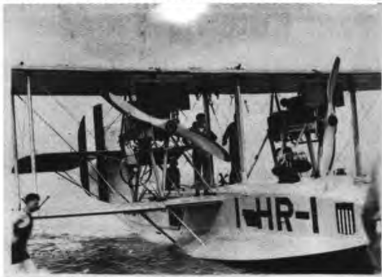
First Hospital Plane, NAS Hampton Roads, VA - 1925.. Note radio-generator with self regulating props with prop-guard rear strut of starboard engine. Paul Koterba standing back of prop.
